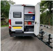
It was fitted by LNB Towbars but is a fairly simple DIY fit (pictorial instructions are available online). When not carrying bikes, the rack can be folded up reducing length, or the swing away portion of the rack can be removed completely without tools, leaving the chassis mounting in place.
